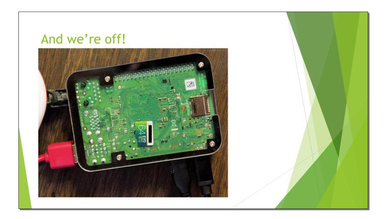
Now that the Pi is assembled and the card is installed, we're ready to go. Well, almost. It's pretty easy to miss the SD slot, and the card gets stuck between the Pi and the case. Shake it until it comes out again. Yes, that's a 64GB card whereas I'm using a 32GB card for the project. There's a lot of bad continuity in this presentation. Spot them all and win a prize! (Not really.)
